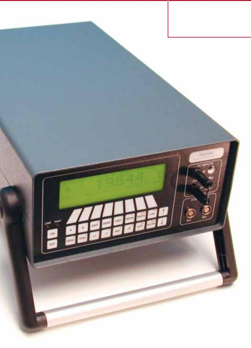
The **Tecal Accu-Temp II** is a high accuracy multi purpose digital thermometer for both platinum resistance thermometers and thermocouples. Dual Channel input allows a probe on Channel B to be calibrated against a standard on Channel A - directly compare any combination of PRT and Thermocouple. The Tecal Accu-Temp II supports 13 thermocouple Types B, E, J, K, N, R, S, T, D, C, I, U, Au/Pt and both 3 and 4 wire 100 ohm Platinum resistance thermometers and RTD's.
